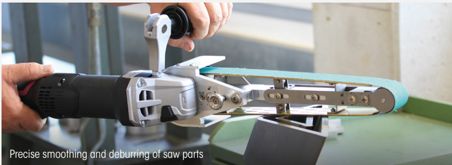
The optional ball joint mount allows the GLADIUS® 1802 HT function as a stationary belt grinder for blade sharpening, etc. (page 227)
